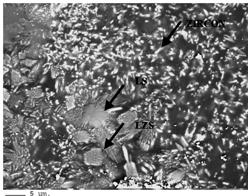
Fig. 4. SEM image of the sintered glassy powders (1 h at 1000 °C).
